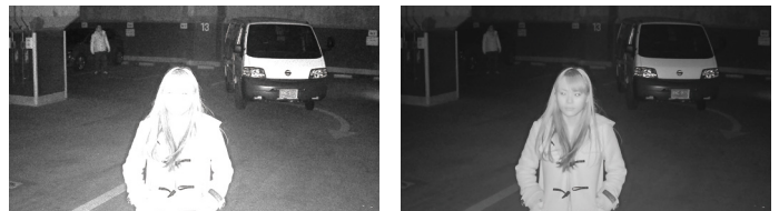
Conventional IR technology (cannot identify close objects due to overexposure) Advanced IR technology (can identify close and distant objects) Actual images
